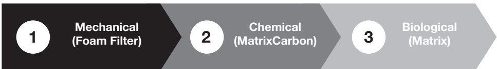
Figure 5: Layering Filtration Media (bottom to top)
